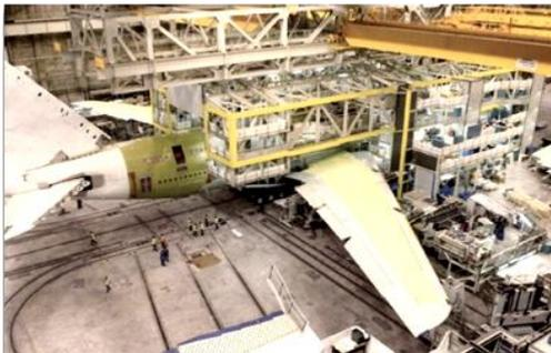
Figure 2a: Field factory with rail guided stationary production of airbus A380
